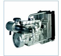
Compliant to Tier 3 / Stage IIIA emissions, the 1106D-E66TA is the latest addition to the common platform concept of 1100 Series diesel engines. Assembled on a new high technology production line, this ultra-clean engine will provide a superior replacement for the 1106C-E60TA Tier 2 / Stage II engine. Frequent computerised checks during the production process ensure high build quality excellence is maintained.
