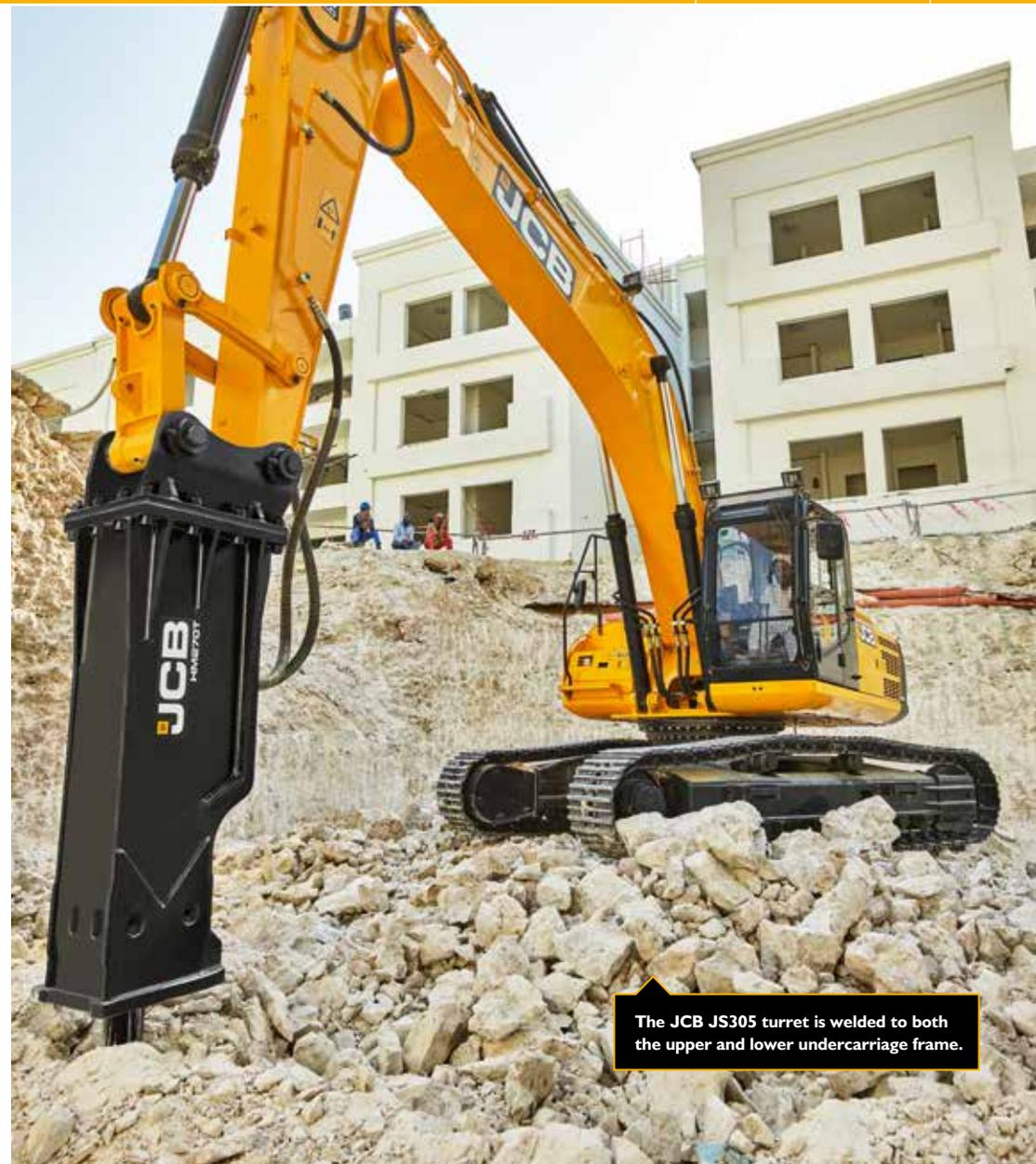
The JCB JS305 turret is welded to both the upper and lower undercarriage frame.
