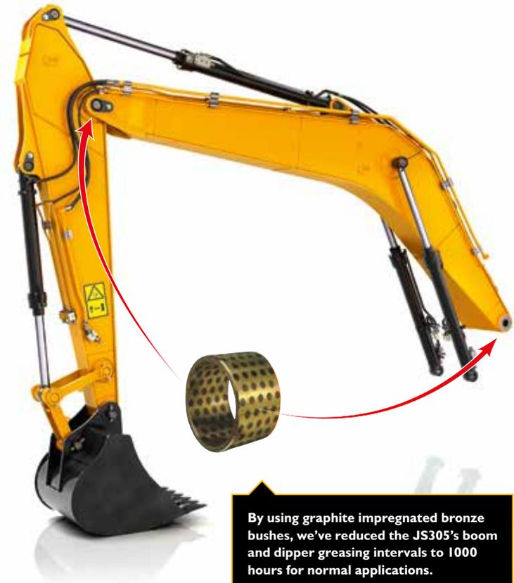
By using graphite impregnated bronze bushes, we've reduced the JS305's boom and dipper greasing intervals to 1000 hours for normal applications.
