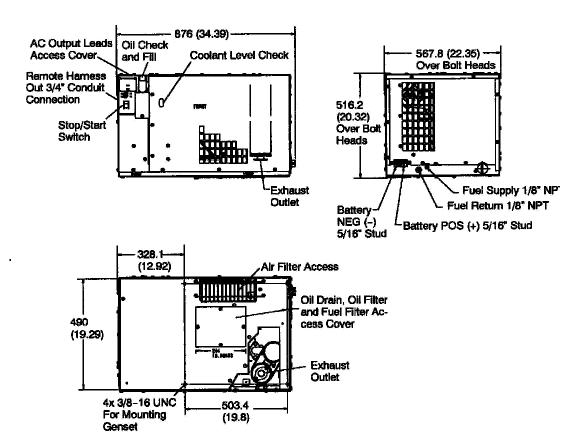
**Note:** This outline drawing is provided for general reference only and is not intended for design or installation. For more information see Operation and Installation manuals or obtain drawing 500-3634 and wiring diagram from your distributor/dealer.
