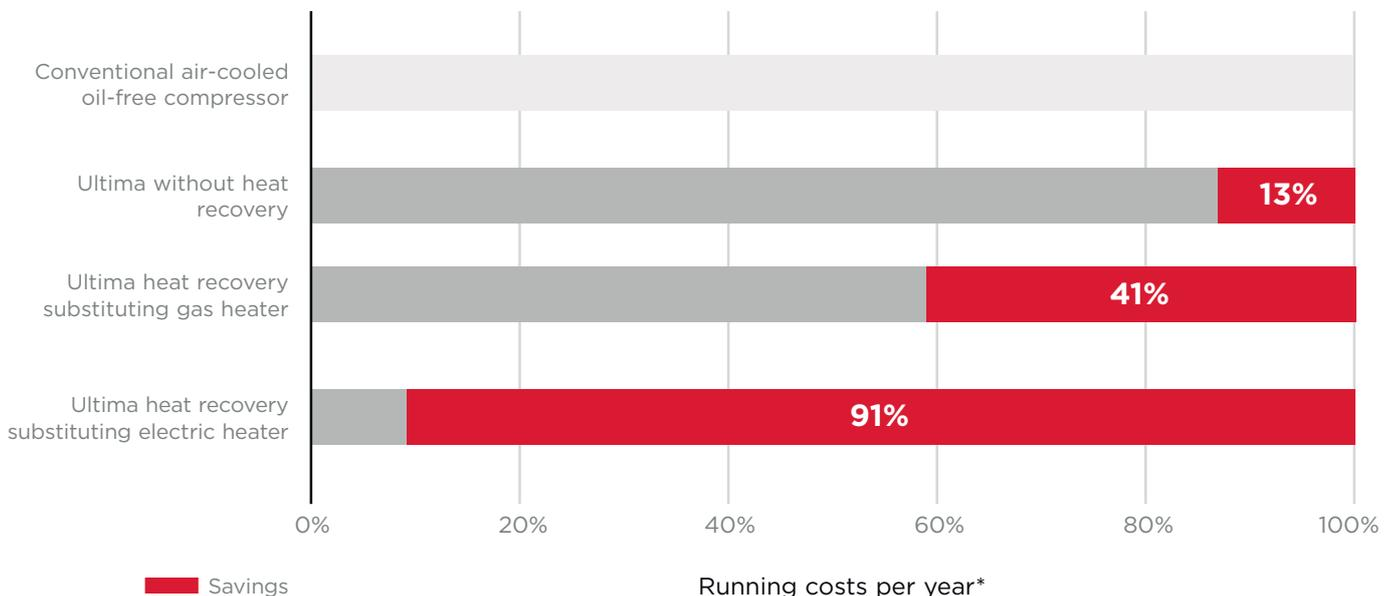
\*Operation @ 20m<sup>3</sup>/min 8 bar, 4,000 hours per year, electricity price 15 ct/kWh, gas price 5 ct/kWh
