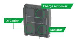
1. Improved cooling performance by changing over to 3 column type structure in a row 2. Easy to clean without disassembling anentire radiator total assembly
