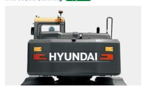
Standard counterweight has been increased by 200kg. This increases stability and lifting capacity.
