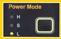
L (Light Power) Mode adjusts engine power and hydraulic torque for optimum performance at improved fuel economy.
